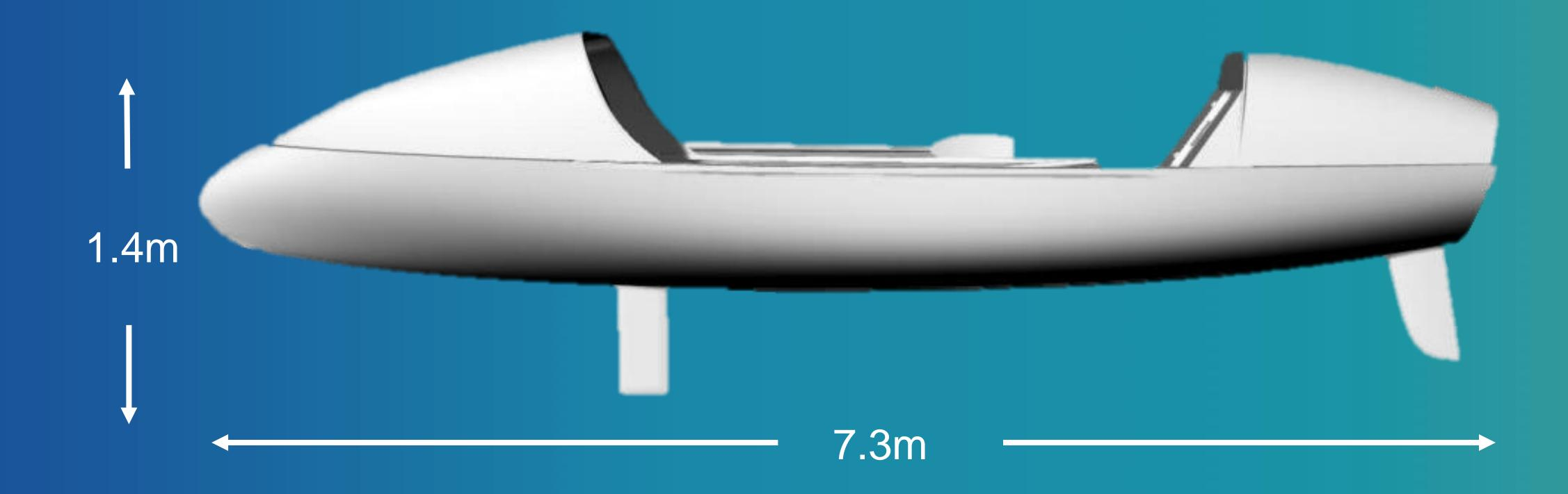
1.4m wide / 1,000kg loaded / fiberglass build / self-righting after capsize
